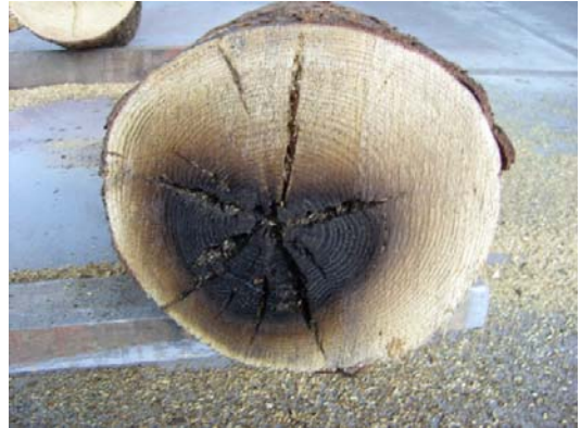
Fig. 4. Runaway phenomenon inside log.
