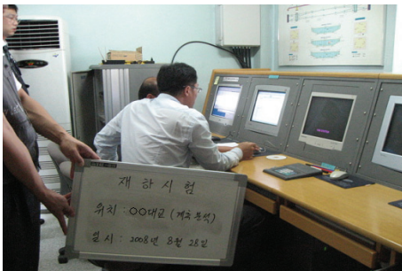
Photo 3 Automatic and semi-automatic calculation of cable force using long-term bridge monitoring system
