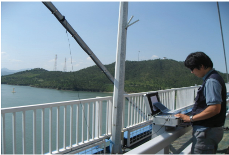
Photo 2 Manual calculation of cable force using portable equipment
