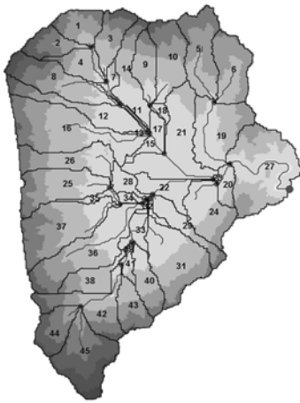
Fig. 4. Subbasins and outlets at the Hae-an watershed.
