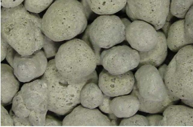
Figure 6. Photographs of the spherical foamed LCD glass.
