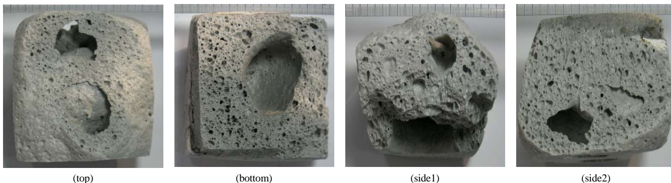
Figure 5. Photographs of the foamed LCD glass block.
