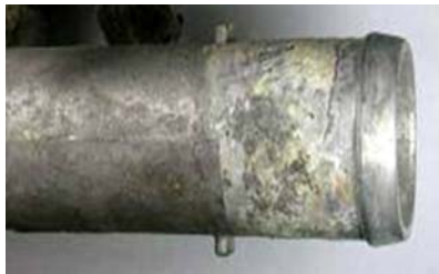
Figure 1. Photograph showing scales and crevice corrosion on the failed thermostat housing.
