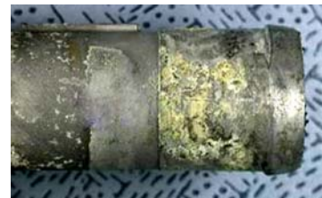
Figure 9. Photograph showing scales and crevice corrosion reproduced by the accelerated test.
