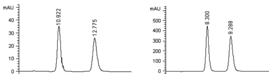
Fig. 1. Chromatograms of enantiomer separation of *N*-FMOC alanine (left) and *N*-FMOC serine (right) using 60%ACN in 0.2% TFA aqueous solution as a mobile phase. See Table 2 for chromatographic conditions.
