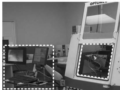
Photo 1 M 3 D system with control electronics outlined in red-dashing, door to environmentally controlled enclosure outlined in yellow-dashing, and computer interface outlined in white-dashing.
