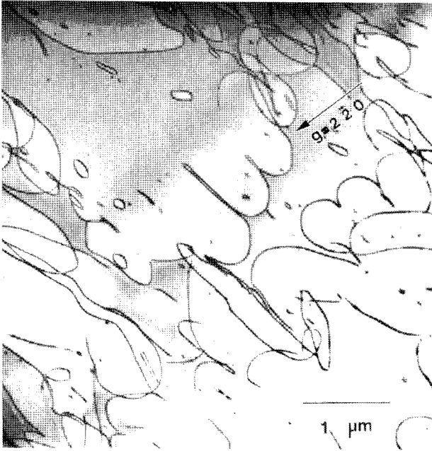
Fig. 3. Dislocation structure at the early stage, B_4 of deformation which showing many dislocation dipoles and prismatic loops.
