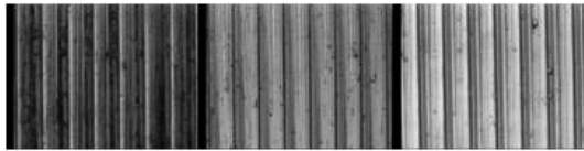
100m/min 200m/min 300m/min (a) Surface shape according to cutting speed (Feed rate 0.08mm/rev, Depth of cut 1.0mm)
