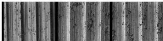
1.0mm 2.0mm 3.0mm (c) Surface shape according to depth of cut (Cutting speed 200m/min, Feed rate 0.197mm/rev)
