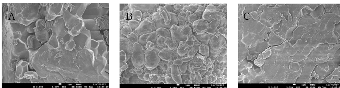
Fig. 1. Scanning electron microphotographs of high amylose rice flours, Goamy (A), Goamy2 (B) and Thailand rice (C) flours, prepared from dry-milling after soaking rice grains.
