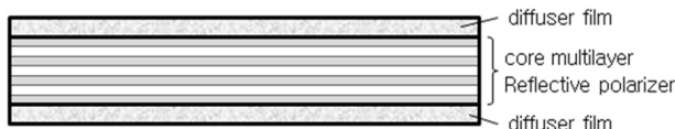
FIG. 2. The internal structure of the reflective polarizer sheet showing the core reflective polarizer with diffuser films attached on the both sides.
