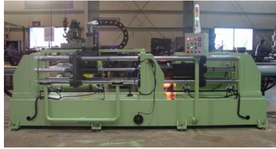
Fig. 9 The manufactured combined drawing machine using 2 hydraulic pumps
