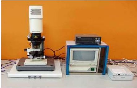
Fig. 5 Measurements setup for characteristic value inspection
