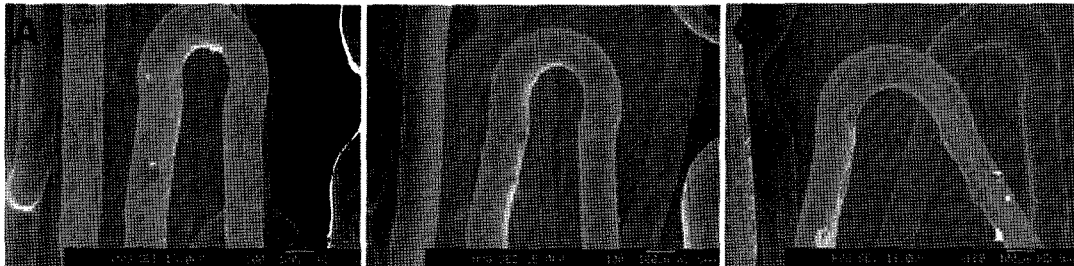
Figure 1. Scanning electron microscopy (SEM) of paclitaxel-incorporated PLCL-coated stents after expansion. (A) 1 wt% PLCL coated stent, (B) 2 wt% PLCL coated stent, and (C) 5 wt% PLCL coated stent.
