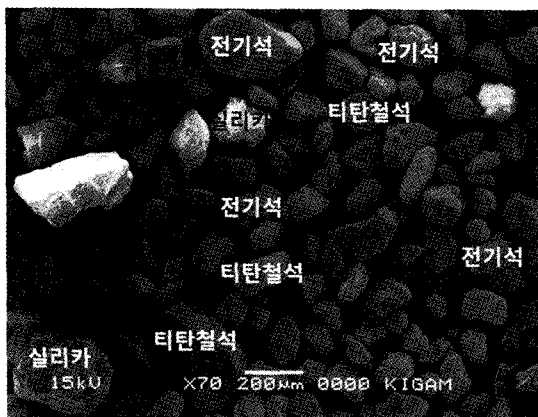
Fig. 5. Scanning electron microscope (SEM) photograph of the magnetic response mineral separated by wet magnetic separation.
