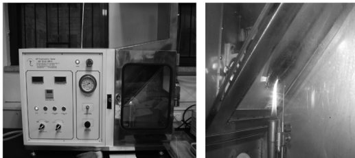
Figure 1. Photograph of 45 degree combustion test apparatus.
