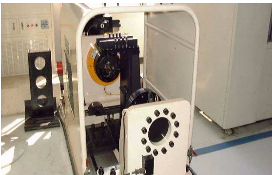
Fig. 5 Photograph of fatigue testing machine
