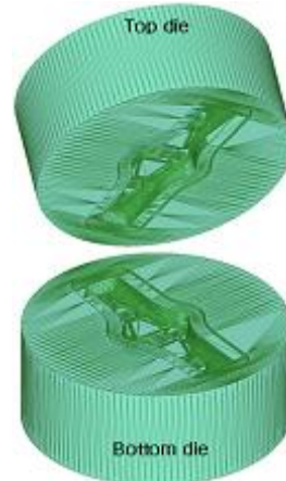
Fig. 4 Die model for forging of yoke
