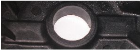
Fig. 11 Flow mark pattern in the two pockets (after improvement)
