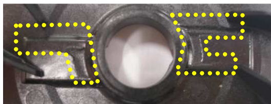
Fig. 3 Flow mark pattern in the two pockets
