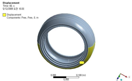
Fig. 6 Fixed Displacement of Tire at Contact with Road Surface
