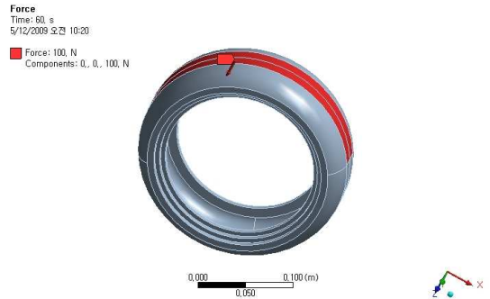
Fig. 5 Applied Load Condition of Tire
