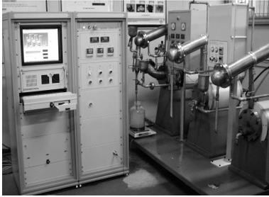
Fig. 2 Indirect heating emulsion pilot system
