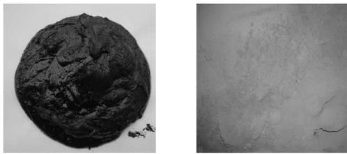
Fig. 8 Sludge and residual sand after emulsion
