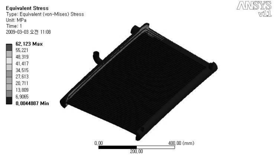
Fig. 11 Thermal Equivalent Stress Contour of Model on Steady State
