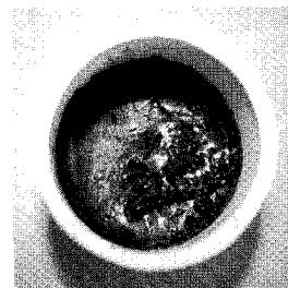
Fig. 9 The state of the half-molten basalt in the crucible
