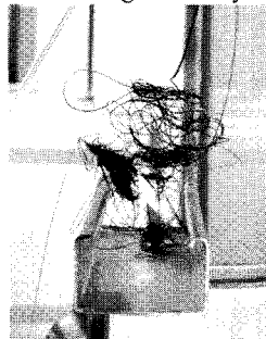
(b) Dripping on the tray due to the low viscosity of the molten
