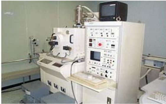
Fig. 1 Focused ion beam (SMI8800, SEIKO, Japan)
