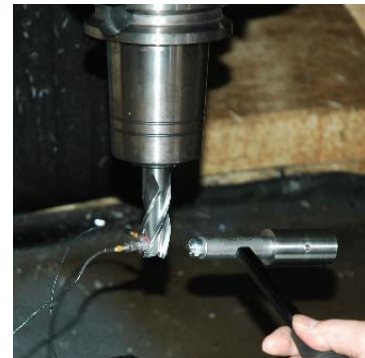
Fig. 4 Measurement of transfer functions using an impact hammer and two accelerometers attached to the machine tool structure
