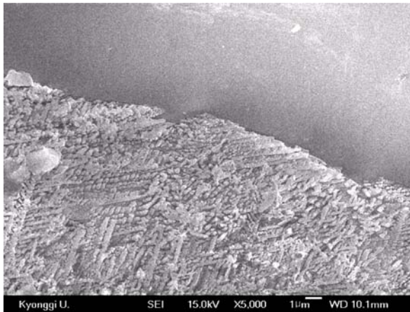
Fig. 4. Enlarged microstructure showing the interface of surface crystal and glassy matrix for glass-ceramics containing 2 wt% TiO 2 (magnified by \times 5,000 ).
