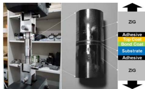
Fig. 8 Experimental setup for bond test
