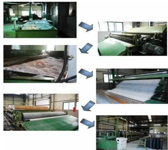
Fig 3. The manufacturing process of nonwoven type mulching.
