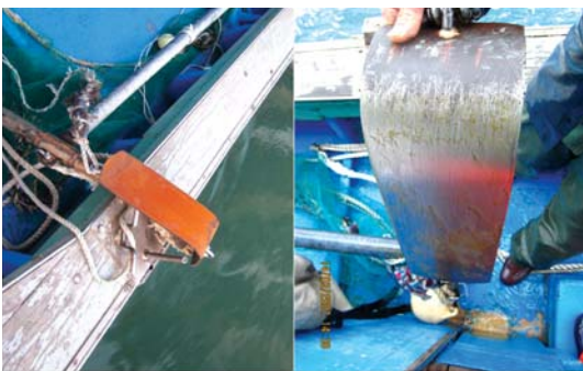
Fig. 4. Changing of detected parts(Ski) of the gear on the seabed after trawling.
