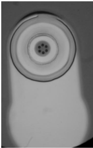
FIG. 3. Microphotography of the PC-VCSEL.
