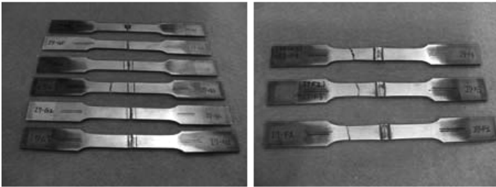
Fig. 11. Picture of Welded INCONEL 718 Alloy. a) Fracture of weld zone (I7-G) and b) Fracture of base metal (I7-F).
