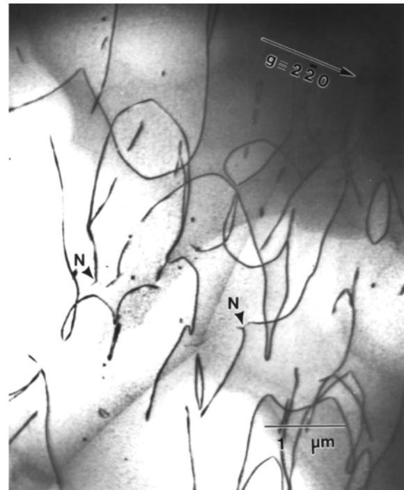
Fig. 6. Dislocation structures on (001) plane of the sample deformed to the stage A_{42} . Most dislocations were edge-type nodes, marked by N.
