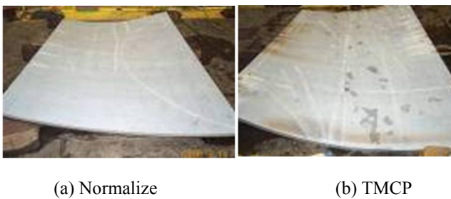
Fig. 2 Density of heating lines for hot forming (Shin et al., 2007) (to same target surface).
