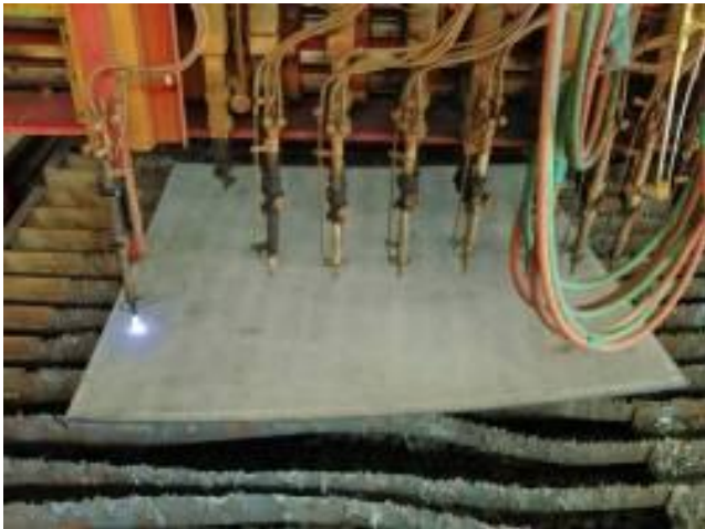
Fig. 15 A heating operation using a gas torch as a heat source.
