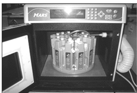
Fig. 1. Microwave accelerated reaction system and pressure sealed vessels used for pretreatment.
