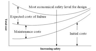
Fig. 1 Selection of reliability index to minimize total cost.
