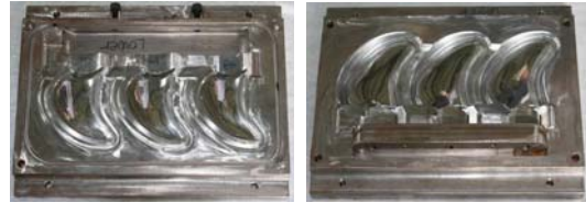
Fig. 6 Molds for blade production
