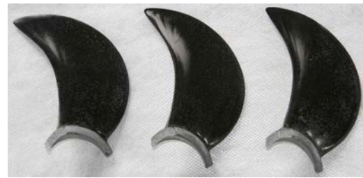
Fig. 7 Blades produced by Glass/Epoxy composite materials
