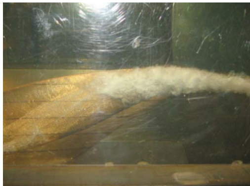
Fig. 9 Cavitation phenomena of large partial blade model at blade angle 43° and cavitation number 0.7 R
