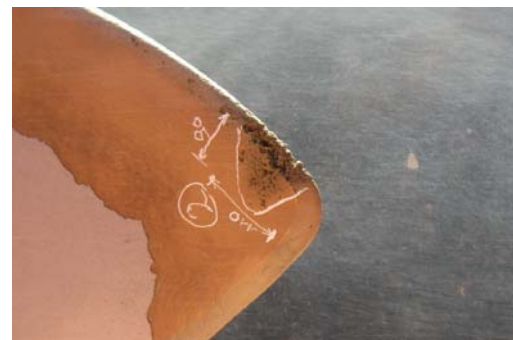
Fig. 2 Blade tip erosion on the propeller of the subject ship
