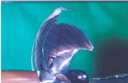
Fig. 8 Cavitation phenomena of model propeller at blade angle 40° and cavitation number 0.7 R
