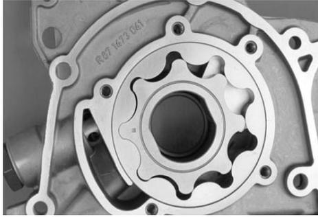
Fig. 1 Real product of Duocentric<sup>®</sup>-IC (TPV, Germany)
