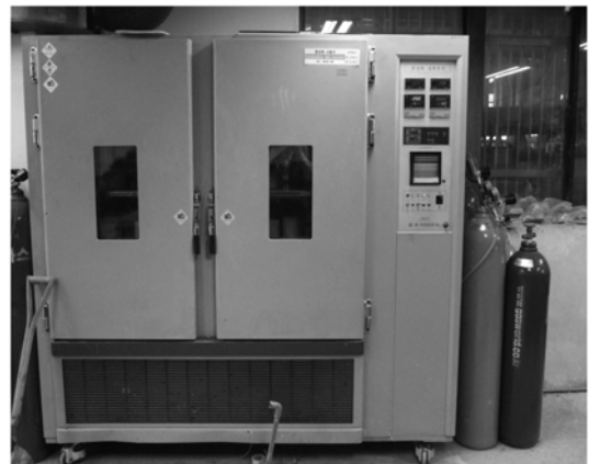
Fig. 1 Carbonation test chamber
