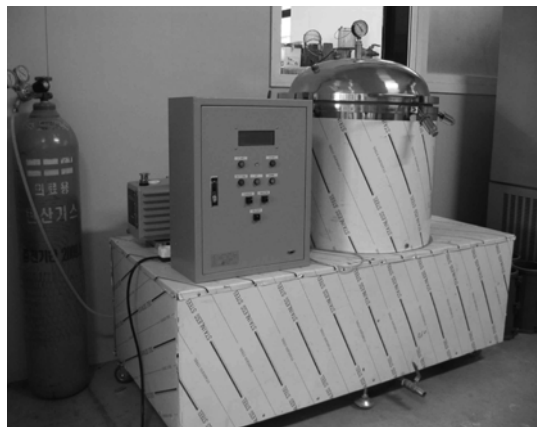
Fig. 2 Accelerated carbonation test chamber
