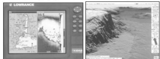
Fig. 29. sounder/chart recorder와 OLEX 3D seabed mapping system
