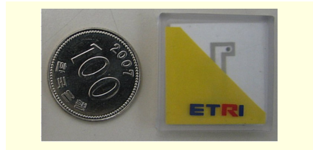
Fig. 6. Photograph of the fabricated tag antenna.
