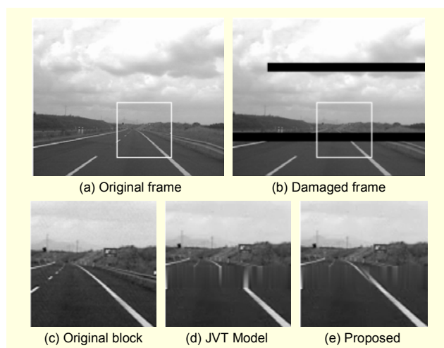
Fig. 16. Comparison of subjective video qualities of the 24th frame of Highway sequence for isolated block error.
