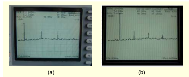
Fig. 5. Measured output spectra of the proposed OSC: (a) before co-design and (b) after co-design.
