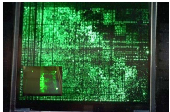
Fig. 10. Operation of a 3.5-inch QCIF AMOLED panel on plastic substrate driven by LTPS TFTs with the mosaic pattern. The inset shows the panel driven to display an "8".
