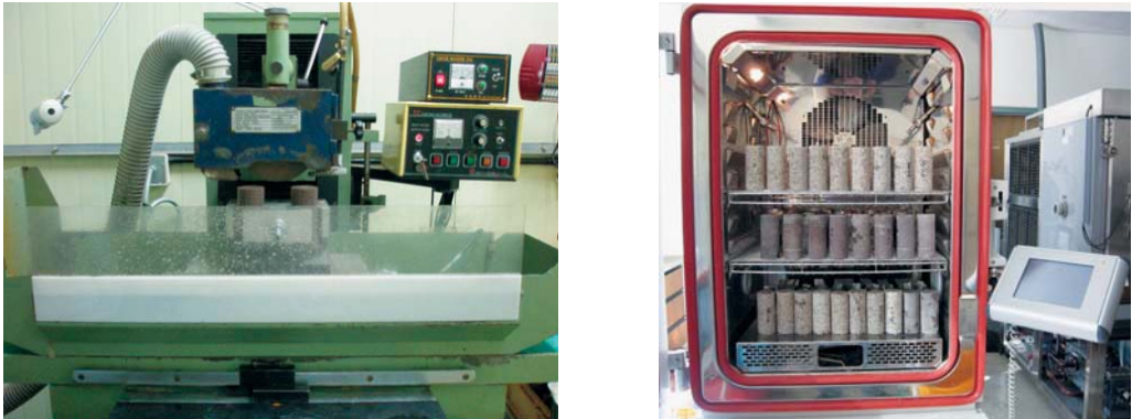
Figure 3. Polishing machine (KSA500-HA) and Freezing-thawing test machine
