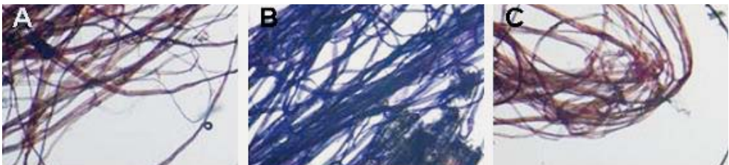
Figure 6. Colorations of Seonseoksa lining paper outside by stains ( A : C-stain, B : Herzberg, C : Wilson's stain)
