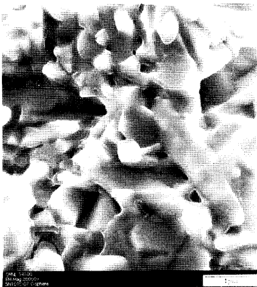
Fig. 10. Flaw type 1 was linked to a surface-located microstructure that had a glassy-like appearance.
