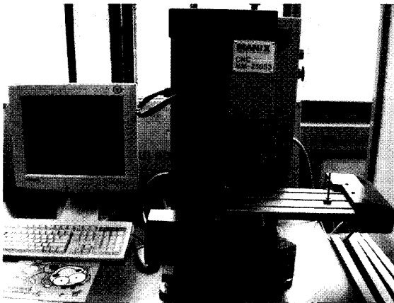
Fig. 2 CNC machine used for incremental forming
