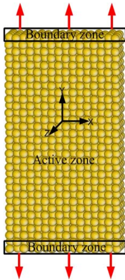
Fig. 3 Boundary condition of simple tension
